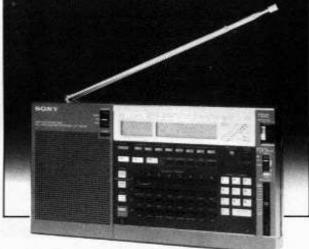
Synchronous demodulators are beginning to be included in a number of commercial receiver designs. An example is this general-coverage AM/FM model by Sony (type ICF2001D): its synchronous demodulator can be switched in to give reduced distortion and fading on AM transmissions, and to enable the user to listen to whichever sideband is less subject to whistles and interference.
